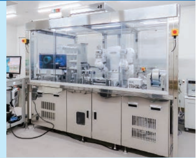
LabDroid "Mahoro," a general-purpose humanoid robot
